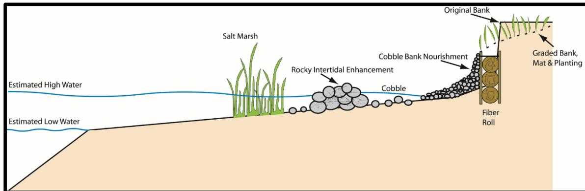
**Figure 3. Preferred alternative of fiber rolls, bank grading, planting, cobble bank nourishment, cobble berm.**
