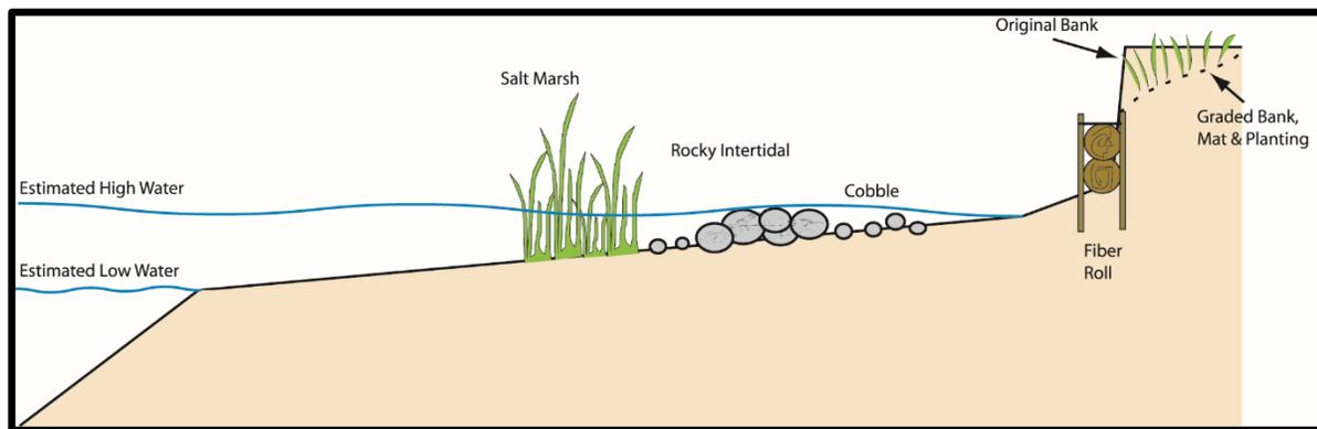
**Figure 2. Fiber rolls installed at the base of the coastal bank.**
